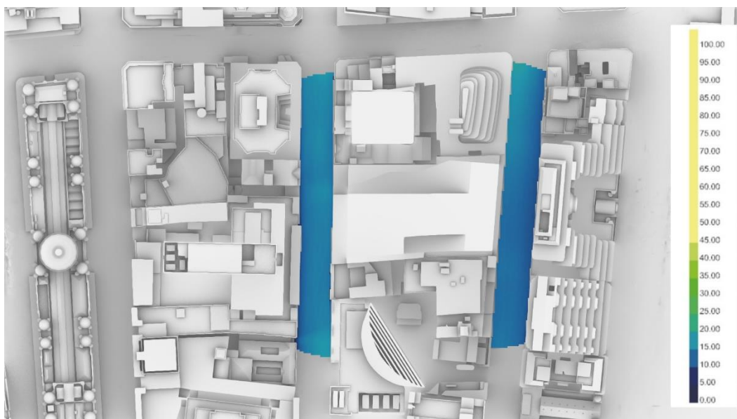
Figure 4.2c Sky View Factor for proposed envelope 6G.
